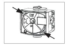
3. Remove the motor plate using the two handles (see arrows).
