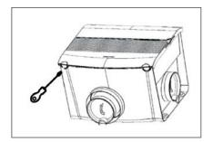
2. Remove the front cover using a flat screwdriver. Behind this cover are the electric wiring, motor and circuit board located.
