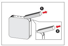
2. Remove the old filter and slide the new filter into the device. Replace the cover.
