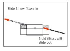
6. Slide three new filter elements into the device on the left side. The old filter elements are automatically ejected from the right side.
