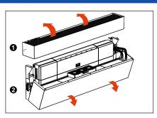
3. Loosen the screws and remove the upper housing from the unit (1). Tilt the lower housing forwards (n.b.: this is held in place with magnets.) Position it in the brackets provided for this purpose (2).
