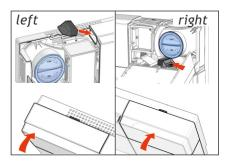
7. Put the two black filter caps (left and right) back in position and close both valves again.
