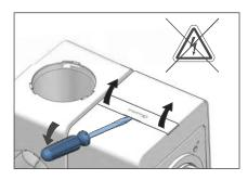
1. Disconnect the power and open the cover of the fan housing using a screwdriver.
