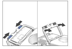
5. Push the two sliders of the bracket toward each other and tilt the bracket upwards to open.
