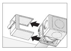
3. Remove the housing by pulling the opened cover upwards.
