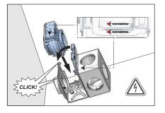
8. Push the fan back into the frame. Squeeze the sliders in the bracket and snap the bracket on both sides to close.
