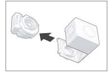
6. Remove the fan from the housing and snap the bracket back into the frame.
