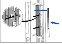
8. Push the three new filters in the sections and press the grille at the bottom with the two clips firmly closed until you feel it snap. Please note that the filter housing must be properly closed for proper operation.
