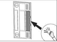
6. Cleaning the air outlet. When the filters do not yet have to be replaced, you can use a vacuum cleaner to clean the filters. You do not need to open the filter housing.
