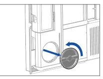
9 . Cleaning the air ducts. Remove the two inspection hatches by turning them to the left and removing them.
