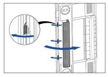
3. Air supply filters. Open the three clips at the left side and tilt the filter housing forwards.
