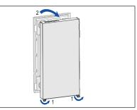
2. Turn the two locking hooks (at the bottom or on the side of the housing). Remove the cover of the Sensa by lifting it upwards.
