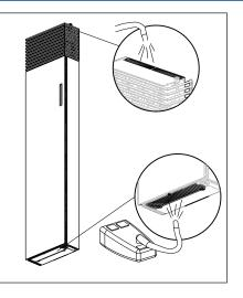
2. Clean the insect mesh at the top and bottom of the unit using your vacuum cleaner.
