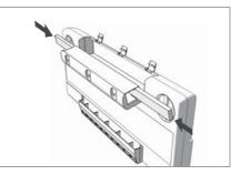
5. Slide the two new filters fully into the filter housing so that they do not project.
