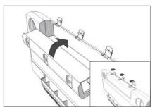
6. Tilt the filter housing upwards and secure with the three clips.
