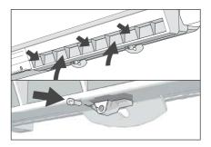
6. Push the three new filters in the sections and press the grille at the bottom with the two clips firmly closed until you feel it snap. Screw the grille in position with the two screws.
