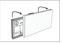
2. Remove the cover of the Sensa by lifting it upwards.
