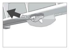
3. Loosen the two screws under the filter cover.
