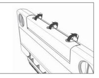
3. Open the three clips on the top and tilt the filter housing forwards.
