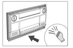
2. Use a vacuum cleaner to remove as much dirt as possible from the filter tray at the bottom.
