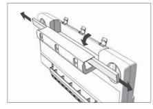
4. Slide the two contaminated filters to the sides out of the fiter housing.
