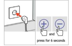
8. Push the plug back into the socket and reset the filter hour counter by simultaneously pressing on the + and - on the display for 6 seconds. The message 'Filter vervuild' will disappear.
