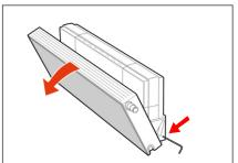
3. Tilt the radiator and, if required, lock it with an Allen key or screwdriver.
