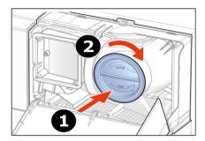
7. Push both blue filter caps fully back in for a correct operation and tighten.
