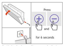
9. Unlock the radiator and tilt it back. Push the plug back into the socket and reset the filter hour counter (by simultaneously pressing on the + and - on the display for 6 seconds ). The message 'Filter vervuild' will disappear. Tighten the locking screws again.
