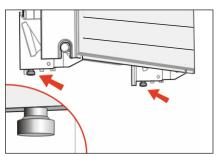
2. There is a locking screw at the bottom of each of the two (or four) radiator consoles. Remove these locking screws.
