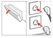
9. Unlock the radiator and tilt it back. Push the plug back into the sockets and tighten the retaining screws.
