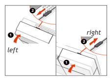
8. Close the covers on the lefthand and right-hand side of the unit, and slide both latching slides outwards.
