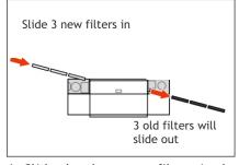
6. Slide the three new filters in the unit from the left-hand side. The old filters will automatically slide out on the right-hand side.
