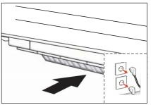
4. Slide the filter tray closed until you hear a clicking sound. Push the plug back into the socket.
