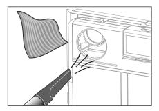
12. Remove any dirt from both channels with a vacuum cleaner or a soft cloth (do not use water).
