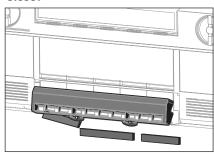
9. Push the filters from the front out of the filter housing. Place the three new filters in the sections.
