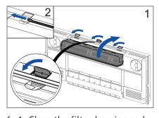
6. 1. Close the filter housing and secure with the three clips. Caution: The filters must not protrude out of the filter housing. 2. Slide the cover to the left to close.
