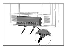
10. Press the grille at the bottom with the two clips firmly closed until you feel it snap. Please note that the filter housing must be properly closed for proper operation.
