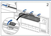
3. Replace the air supply filters. 1. Slide the cover to the right; the clips are now visible. 2. Open the three clips on the top and tilt the filter housing forwards.
