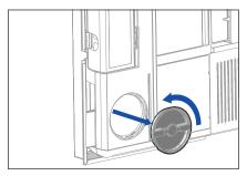
9. Cleaning the air ducts. Remove the two inspection hatches by turning them to the left and removing them.
