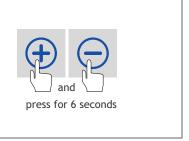
15. Reset the filter hour counter by simultaneously pressing on the + and - on the display for 6 seconds. The message 'Filter vervuild' will disappear.
