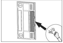
6. Cleaning the air outlet. When the filters do not yet have to be replaced, you can use a vacuum cleaner to clean the filters. You do not need to open the filter housing.
