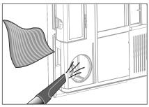
11. Remove any dirt from both channels with a vacuum cleaner or a soft cloth (do not use water).
