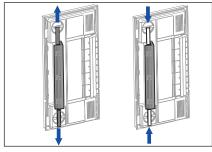
4. Replace the two dirty air supply filters through the top and the bottom of the filter housing.
