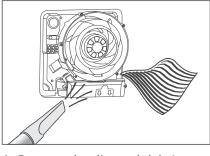
6. Remove the dirt and debris with a soft, lint-free cloth or vacuum cleaner.
