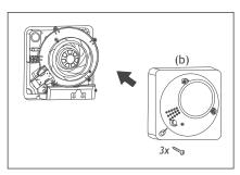
8. Install the inner housing (b) on the ClimaRad Fan. Tighten the 3 screws.
