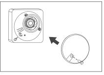
9. Replace the cover and tighten the locking screw.
