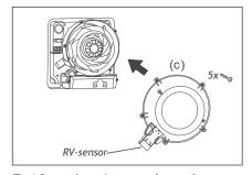
7. After cleaning, replace the cover (c) and reconnect (if present) the RV sensor.
