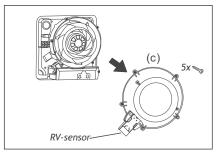
5. Disconnect (if present) the RV sensor and remove the 5 screws of the boiler cover (c).
