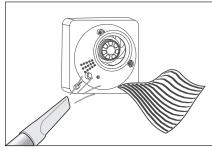
3. In the event it is only slightly dirty the dirt and debris can be removed with a soft, lint-free cloth or vacuum cleaner.
