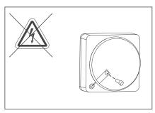
1. Disconnect the power in the electrical box and remove the locking screw.
