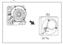
4. In the event it is very dirty the three screws of the inner housing (b) must be loosened and the inner housing removed.
