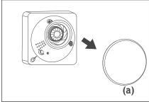
2. Remove the round cover (a) by pulling it off and inspect the fan for dirt.
