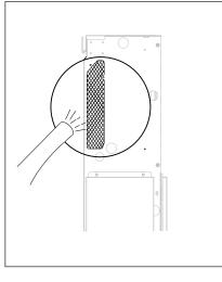
5. Clean the insect mesh on both sides of the convector using your vacuum cleaner.
