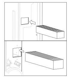
4. Remove both polluted filters and place the new inlet filter (below) and output filter (above).
